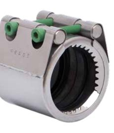
AVK's range of Repico<sup>®</sup> couplings in stainless steel 316 comprises tensile "Grip" couplings for all metal pipe materials up to DN400, and non-tensile "Slip" couplings for all pipe materials up to DN2000. Repico<sup>®</sup> couplings are suitable for water and wastewater applications.
