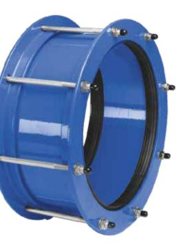
AVK's range of fabricated fittings comprises non-tensile straight couplings, step couplings and flange adaptors in DN350-2000. The range is suitable for ductile and grey cast iron, steel, uPVC and GRP pipes for water and wastewater applications up to 25 bar.
