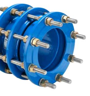
AVK dismantling joints provide easy installation and disassembly of flanged pipework and equipment and compensate for axial displacement of the pipe during installation and dismantling. The range is available in DN40-2600 in PN10/16 and up to DN1200 in PN25.
