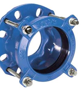
The AVK Supa<sup>®</sup> universal straight couplings, step couplings and flange adaptors are suitable for uPVC, cast iron, ductile iron, steel and AC pipes. The couplings range from DN40 to 400 and are suitable for water and wastewater applications.
